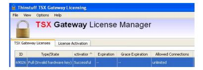
For virtual machines, this case occurs, when the MAC-address of the primary Windows network interfaces has changed.
